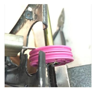
1. Cut end of threaded rod as shown to half the thickness of a standard jigsaw blade
