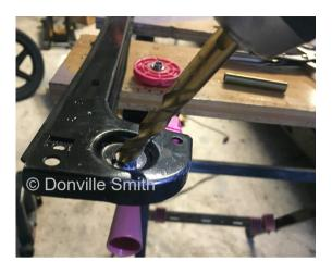
2. Make hole slightly wider than drill bit
