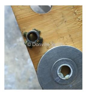
3. Insert hollow fastener into spacer and place into pulley wheel
