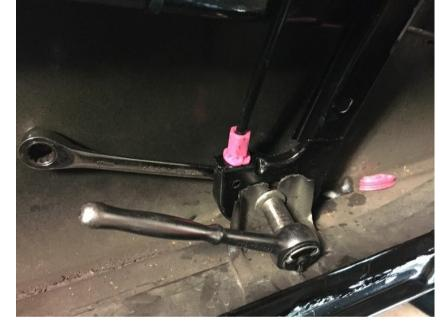
Tools needed to affix pulleys to regulator frame:
