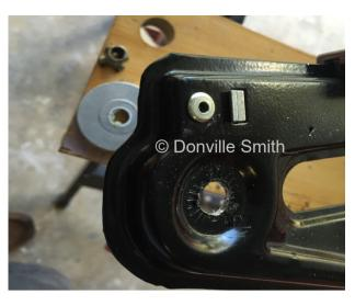
2. Make hole wide enough for hollow fastener to fit without being too loose
